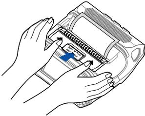
With a roll of stock installed, slide the peeler body towards the back of the printer.
