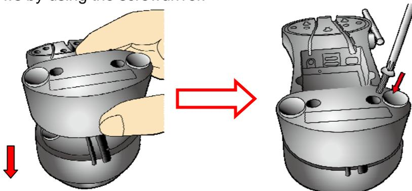
Step 3: Push up and shift out the wedge and then inversely insert the wedge. Note that the protruding portion is upward.
