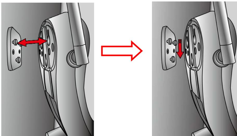
Step 6: The cradle wall-mount installation is completed, as shown in the figure below.
