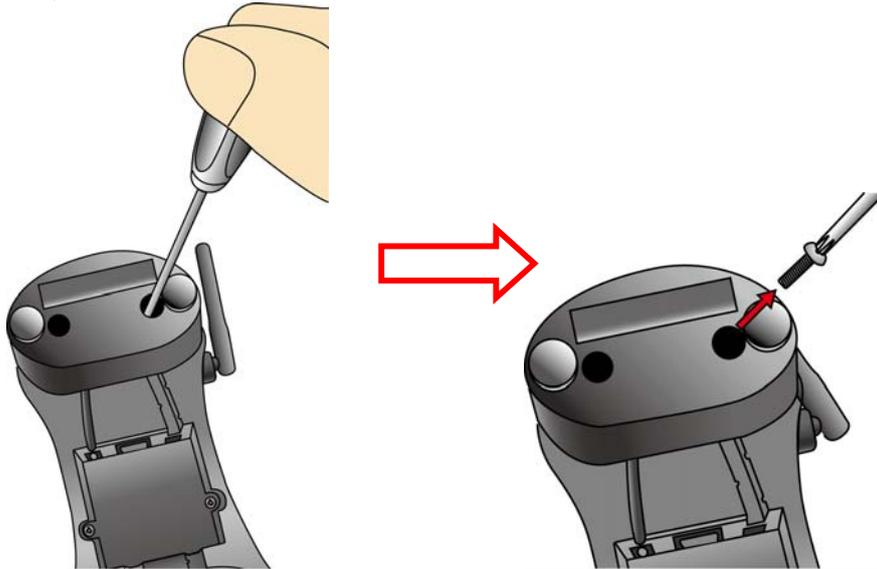
Step 2: Move the stand of cradle to the lower portion of the cradle from the upper portion adjacent to the antenna. Then, secure the stand to the cradle with 2 screws by using the screwdriver.
