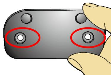
Step 5: Align the two holes on the bottom surface of the cradle respectively with the two short pillars of the iron plate for insertion of the pillars into the holes. Then, push the cradle downwards to wedge the pillars into the guidance groove.
