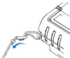
After pulling out the end of strap tightly, put it into the clip to be fastened.
