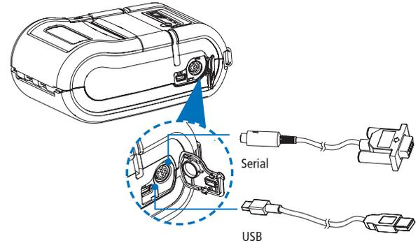
1. Connect USB or Serial cable into the cable connector on the printer.
