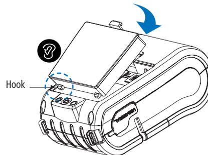
1. Align battery hook as shown in the picture
