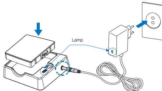
1. Insert the battery into the battery holder as shown above
