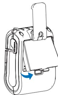
Remove the battery as shown
