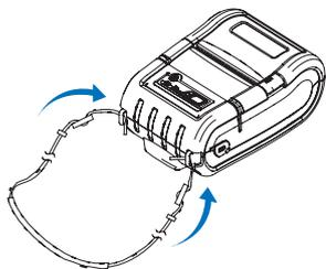
Insert the strap into the hook on the printer.
