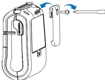
Tighten the screw with driver as shown.
