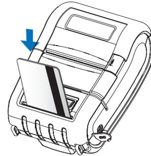
Insert the card in the direction of the arrow as shown in the picture.
