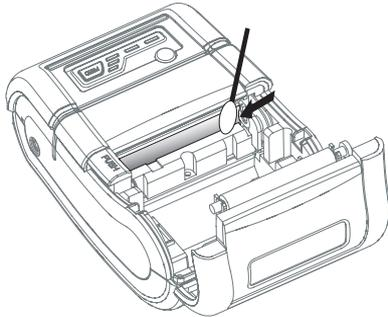
1. Use an applicator swab moistened with an alcohol solution to clean the print head and remove any dusts.
