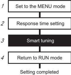
\* Steps 1, 2 and 4 are not required when the response time setting is completed since smart tuning can be performed even in the RUN mode.
