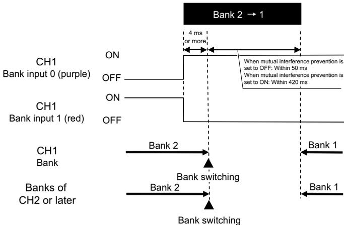
(\*) Bank input is executed by the ON/OFF combinations of CH1 BANK input 0 and CH1 BANK input 1 when connecting two or more Amplifier Units.
