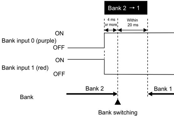
(\*) Bank input is executed by the ON/OFF combinations of BANK input 0 and BANK input 1.
