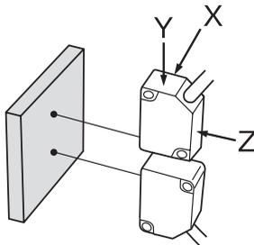
**Results: For all models, the distance that causes malfunction is 0 mm in all the X, Y, and Z directions.**
