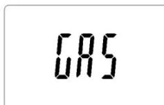
The operation of the transmitter is disabled. Place the throttle stick at idle to allow the transmitter to continue its initialization sequence and become fully operational.
