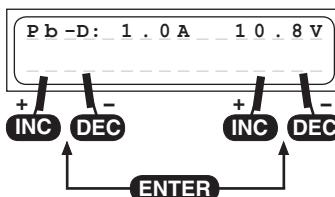
The typical purpose of this program is to determine the residual capacity of a drive battery.
