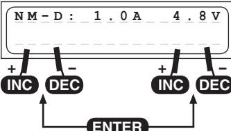
The typical purpose of this program is to determine the residual capacity of a transmitter, receiver or drive battery, or to discharge the pack to a defined level.
