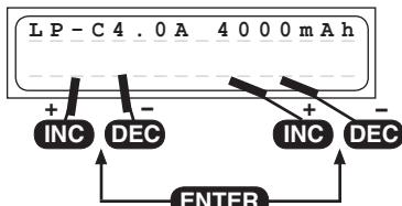
This program charges the battery using the capacity (charge current) which you set.
