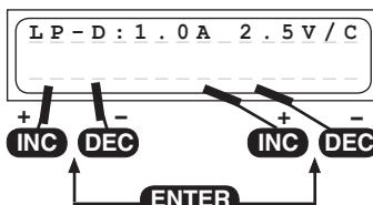
The purpose of this program is to determine the residual capacity of a Lithium pack which has not been fully discharged.
