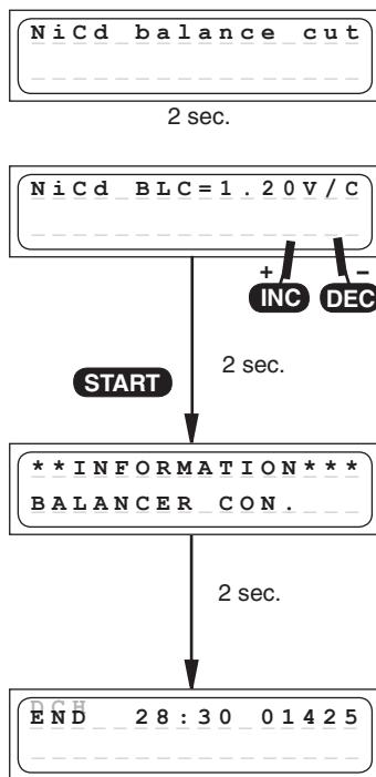
The discharge balancing program does discharge and balance up to 8 cells of a battery pack.
