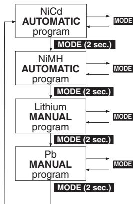
In the interests of clarity, the charge and set-up facilities of the ULTRA TRIO PLUS 16 are divided into four logical program groups. A separate program group is provided for each of the different battery types: **Nickel-Cadmium**, **Nickel-Metal-Hydride**, **Lithium-Ion / Lithium-Polymer / LiFePO<sub>4</sub>** (LiFe) and **Pb** (lead-acid) batteries.
