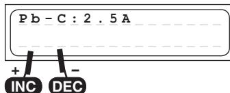
If the battery manufacturer states a low maximum charge current, then it is important to limit the charge current to that value to avoid the charger setting a higher current if the battery appears to be willing to accept charge.
