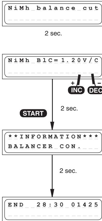
The discharge balancing program does discharge and balance up to 8 cells of a battery pack.
