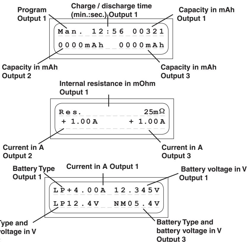
The two-line liquid-crystal screen displays in a clear form the important information generated during the charge / discharge process. The information remains visible on-screen until you disconnect the battery that is being charged. Once you connect another battery for charging, the previously displayed values are erased, and cannot be called up again.
