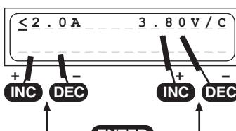
This program does charge or discharge the battery to the best storage voltage.
