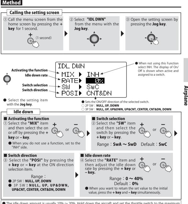
• The idle down amount is usually 10% ~ 20%. Hold down the aircraft and set the throttle switch to the maximum slow position while the engine is running and adjust the idle drop amount while turning the switch on and off.
