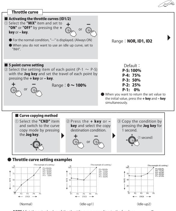
**NOTE**: Set the actual value of the throttle curve according to the fuselage specifications.
