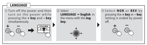
Return from the transmitter setting screen to the normal menu by turning on the power without pressing a key.
