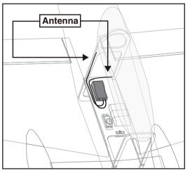
This is not a critical figure, but the most important thing is to keep the antennas away from each other as much as possible.
