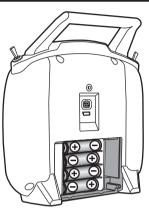
Load the new AA size batteries. Pay very close attention to the polarity markings and reinsert accordingly.
