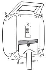
Slide the battery cover back onto the case.
