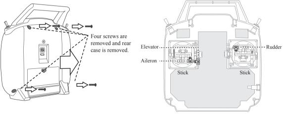
Mode 2 transmitter with rear case removed.
