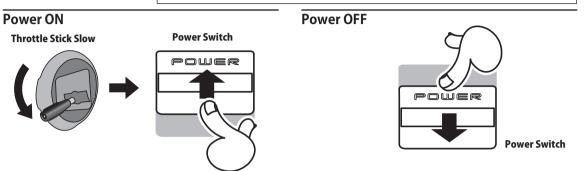
If the power switches are turned off in the opposite order the model may unexpectedly run out of control and cause a very dangerous situation.
