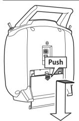
Slide the battery cover off the transmitter in the direction of the arrow in the figure.
