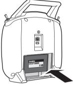
Insert the connector of the new battery and load the new battery into the transmitter.
