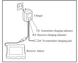
According to the description of the battery to be used and its exclusive charger, please use it after carrying out full charge.
