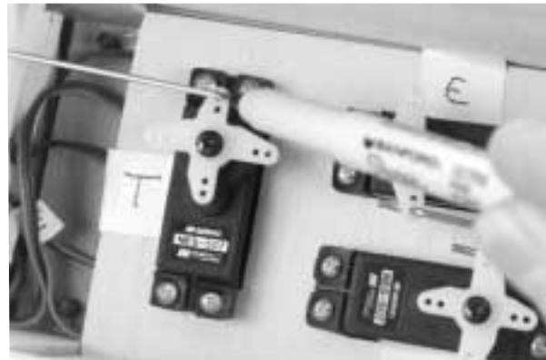
**36.** Using z-bend pliers, make a z-bend at the marked spot on the rod and cut off the excess rod.
