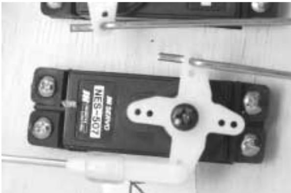
**42.** Be sure the rudder servo is centered. Using a felt tipped pen, place a mark on the **unthreaded** end of the steering pushrod where it passes the nose wheel steering arm.
