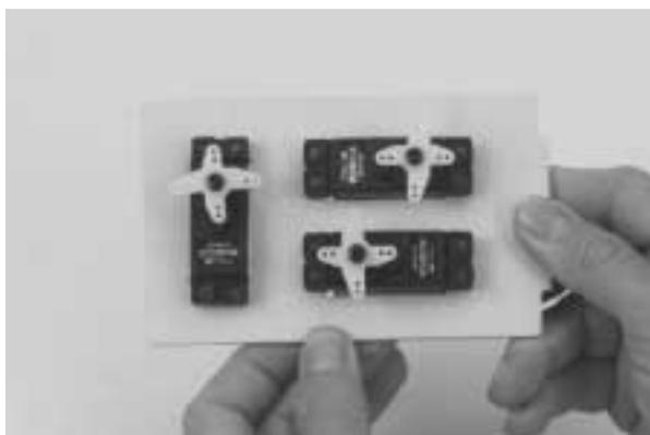
**3.** After the proper servo fit has been achieved, remove the three servos from the servo tray. Trial fit the servo tray into the fuselage, noting the correct orientation. The single servo cut-out should be closest to the front of the fuselage.
