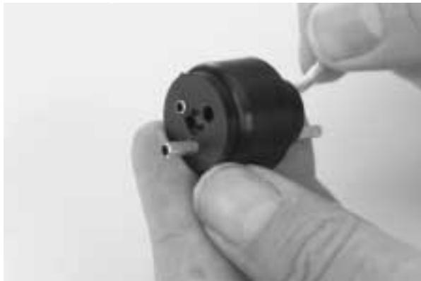
5. Slide the two black plastic caps over the aluminum tubes as shown, noting the orientation of the caps. The small inside cap and the “bumps” face away from the black rubber stopper. The large outside cap and the “bump” go away from the black rubber stopper.
