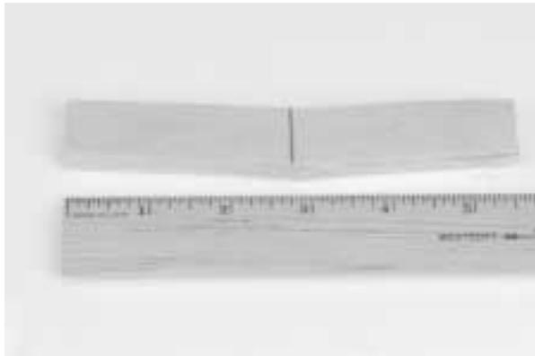
**7.** Trial fit the dihedral brace, or wing joiner, into one of the wing panels. It should insert smoothly up to the center line marked in Step 6. Now slide the other wing half onto the dihedral brace until the wing panels meet. If the fit is overly tight, it may be necessary to lightly sand the dihedral brace. Check to see if the alignment of the wing is accurate.
