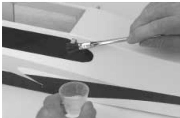
**4.** If necessary, wipe away the excess epoxy using a paper towel and rubbing alcohol, being careful not to disturb the alignment of the wing dowels.
