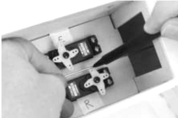
**22.** Using z-bend pliers, make a z-bend at the marked location on the rod. Cut off the excess rod.
