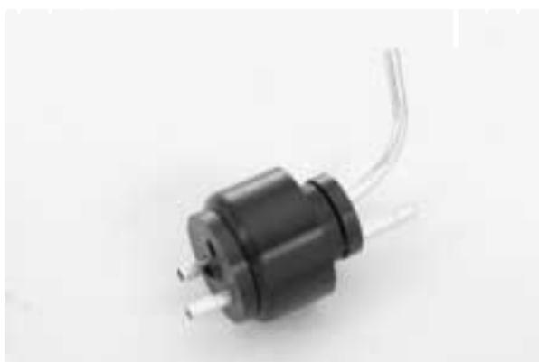
6. Locate the silicone fuel tubing and the metal clunk. Insert the fuel clunk into one end of the fuel tubing. This assembly will be used for the fuel pickup inside the fuel tank.
