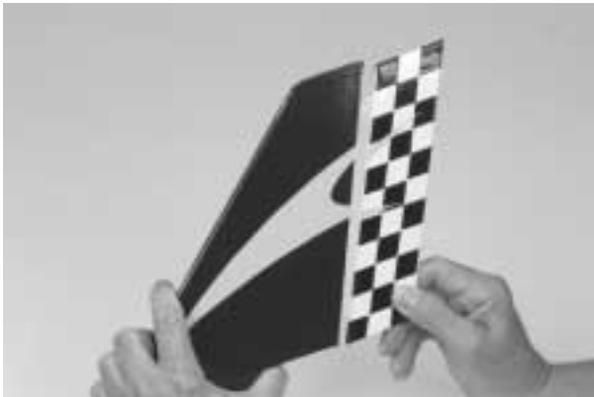
**2.** Remove the three hinges from the rudder and flex them along the hinge line so they move freely.
