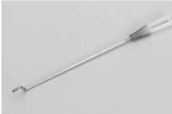
**7.** Install the z-bend into the outermost hole on either side of the servo arm.
