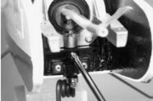
**6.** Attach the nose wheel to the nose gear strut and hold in place with a plastic spacer from the plastic parts tree, a 5/32" wheel collar and a 3mm screw. Be sure to secure the screw with thread lock.
