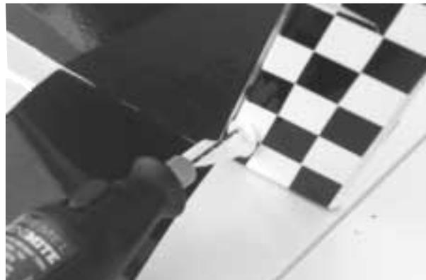
**9.** Install the rudder control horn using the screws and back plate provided.
