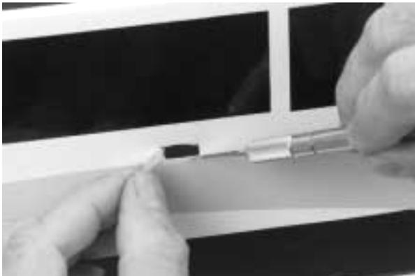
**9.** Detach the switch plate from the receiver switch harness. Center the switch plate over the hole cut in the previous step. Using a felt tipped pen, mark the screw holes on either end of the switch plate.
