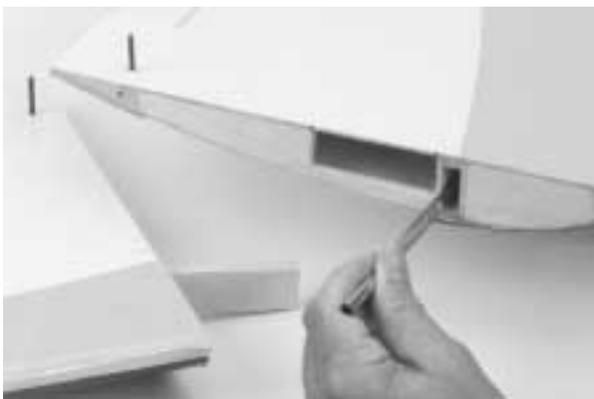
**15.** Smear epoxy on all sides of the exposed area of the dihedral brace and uniformly coat both wing roots with epoxy.
