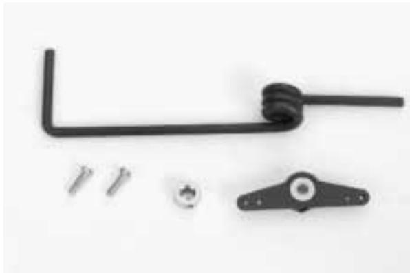
**2.** With the screw hole facing forward, slide the nose gear control horn onto the straight end of the nose gear. Note the orientation as shown below.
