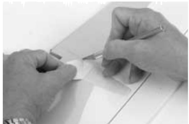
**8.** Mix approximately 1/8 ounce of 30-minute epoxy to install the horizontal stabilizer. Using an epoxy brush or mixing stick, spread epoxy onto the bottom of the horizontal stabilizer along the area where the covering was removed in the previous step and to the fuselage where the horizontal stabilizer mounts.
