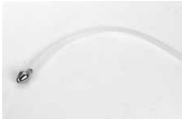
7. Install the open end of the fuel tubing on the shorter aluminum tubing.
