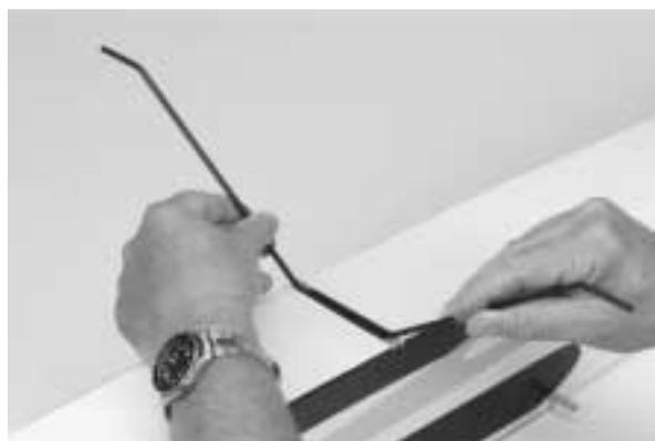
**4.** Remove the two landing gear straps from the plastic parts tree and place them across the landing gear struts so they are evenly spaced on the landing gear. Using a felt tipped pen, mark the location of the two landing gear mounting strap holes.
