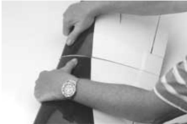
**Note:** It's a good idea to place a sheet of waxed paper under the center joint of the wing so any excess epoxy doesn't adhere to the surface of the work area. Use rubbing alcohol and a paper towel to wipe off any excess epoxy.
