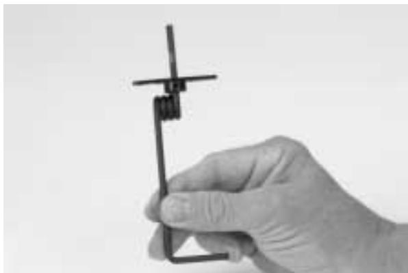
**3.** Place a 5/32" wheel collar on the nose gear. Insert the nose gear into the nylon nose gear mount. Insert the nose gear steering arm onto the nose gear between the nylon motor mount and metal motor mount as shown. Insert until the coil is just below the bottom of the fuselage.
