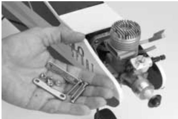
**3.** Place one engine mounting bracket across each of the engine mounting lugs as shown.
