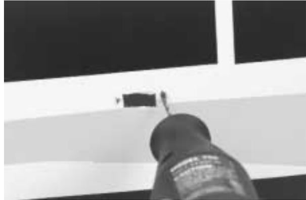
**11.** Reposition the switch plate as shown and place the switch on the inside of the fuselage. Using the two screws supplied with the switch, attach the switch to the fuselage. The suggested orientation of the switch is to have the "on" position forward and the "off" position toward the back.
