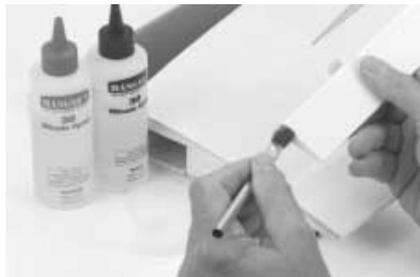
**5.** Wipe off any excess epoxy using a paper towel and rubbing alcohol.
