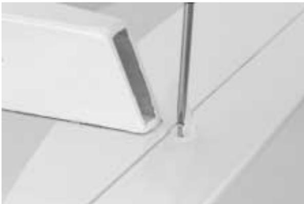
**6.** Turn the fuselage over so it's resting upright. Measure up 1/2" from the bottom of the rudder and mark with a felt tipped pen. This mark will serve as the center of the rudder control horn.
