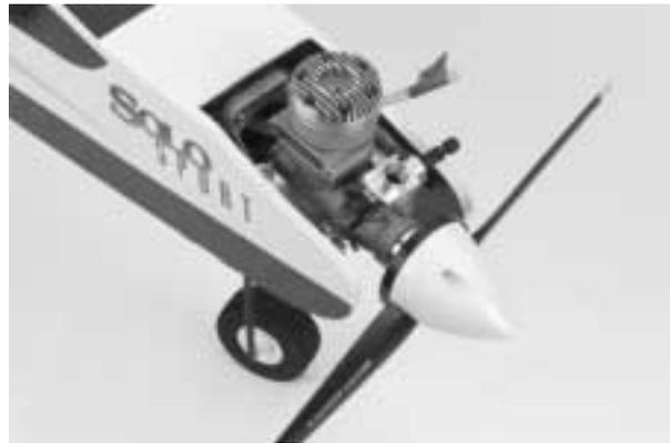
**2.** Install the spinner back plate on the engine crankshaft. Place the propeller on the crankshaft and position it so it seats correctly against the spinner back plate. Next, install the engine washer and the prop nut onto the crankshaft and tighten securely.
