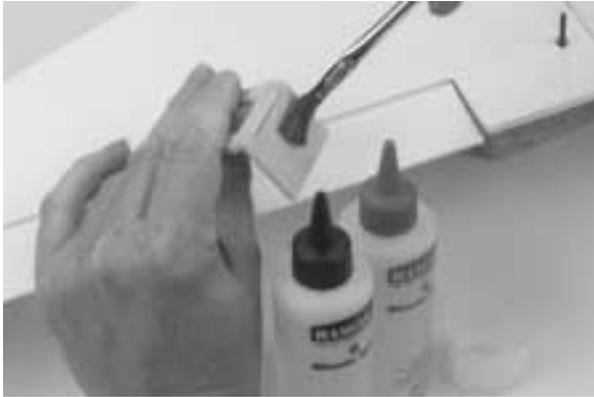
**14.** Locate the wing center tape and remove the adhesive backing. Starting at the rear of the aileron servo tray, wrap the tape completely around the wing joint seam to the rear of the servo tray. Gently pulling on the tape while pressing it down onto the wing will provide a smooth seam. Cut off any excess tape with a pair of scissors.
