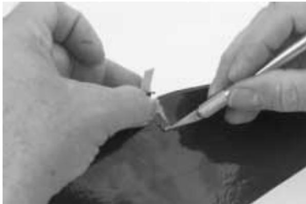
**2.** On the rear of the fuselage, slots are pre-cut for the vertical stabilizer and the rudder pushrod exit. Using a sharp hobby knife, carefully cut out the opening for the vertical stabilizer. The opening for the rudder pushrod will be cut out later in Section 15, Step 18.
