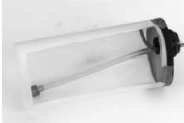
**9.** Select two of the longer pieces of music wire and insert both into the fuselage through the hole in the firewall. Do not insert all the way. These pieces of music wire will serve as guides for passing the fuel tubing attached to the fuel tank stopper into the fuel tank compartment when installing the fuel tank.
