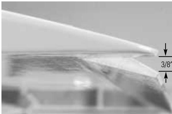
3. If the ailerons do not move in the correct direction, switch the aileron servo reversing switch on the transmitter.
