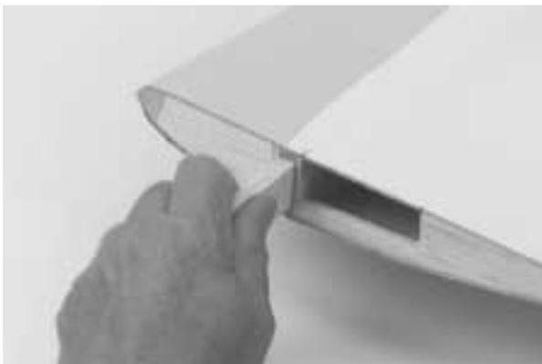
**14.** Apply a generous amount of epoxy into the wing cavity of the other wing half.
