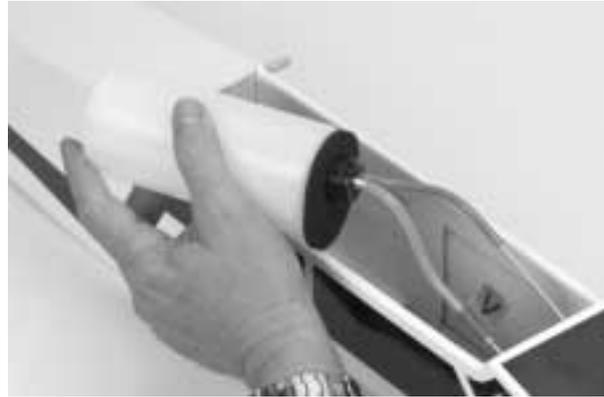
**13.** Press the fuel tank firmly against the firewall until the stopper inserts into the hole in the firewall. The rubber stopper of the fuel tank will be nearly flush with the firewall. The fuel tank should fit snugly into the compartment held in place by friction against the fuselage formers.
