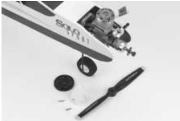
**3.** Attach the spinner to the spinner back plate using the two screws provided in the hardware bag.
