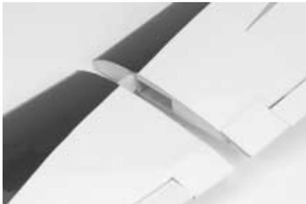
**8.** Now check for the correct dihedral angle. To do so, place the wing on a large, flat surface (with the aileron rods hanging off the edge) with one wing panel resting on the surface; the opposite wing tip should be exactly  $4\frac{1}{2}$ " from the surface (see illustration below). A good point to measure from is where the plastic wing tip joins the end of the wing panel. If the angle
