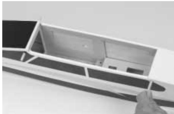
**3.** Mix a small amount, approximately 1/4 oz., of 6-minute epoxy. Using an epoxy brush, apply a thin coat of epoxy to the wing dowels as shown to prevent the dowels from becoming fuel-soaked during flight. The epoxy will also prevent the dowel from moving in the holes.
