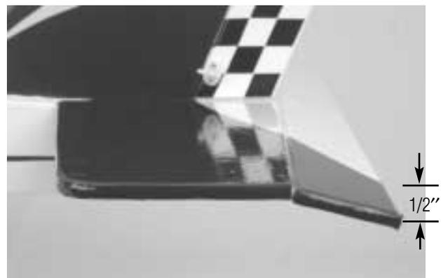
7. If the elevator moves up, switch the elevator servo reversing switch on the transmitter.
