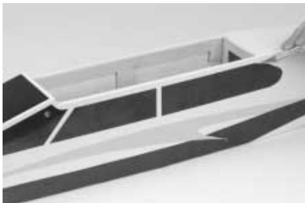
**2.** Insert one of the wooden dowels into each of the wing dowel holes, making sure that an equal amount of dowel extends from each side of the fuselage.
