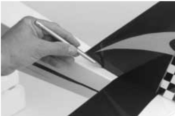
**13.** Remove the vertical stabilizer from the fuselage. Using a sharp hobby knife, carefully cut away the covering below the lines drawn in the previous step. Do **not** cut into the balsa wood as this will affect the structural integrity of the stabilizer.
