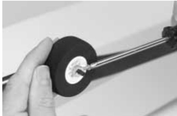
**6.** Reposition the two main landing gear struts and the landing gear mounting straps. Using the four 2.6mm self-tapping screws from the hardware bag, fasten the landing gear to the bottom of the fuselage as shown.
