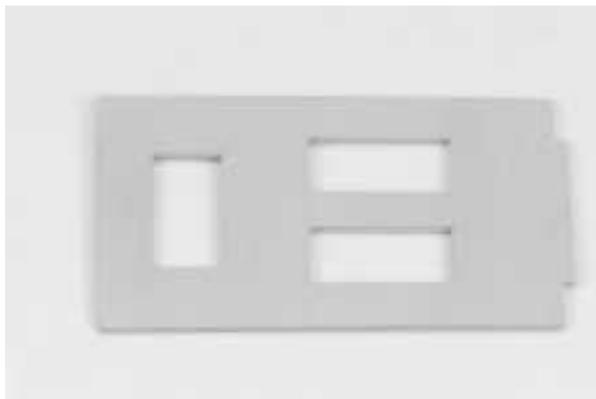
**2.** Trial fit the throttle, elevator, and rudder servos into the servo tray. Depending upon the servos used, it may be necessary to enlarge the openings of the tray slightly using a file or a sharp hobby knife.
