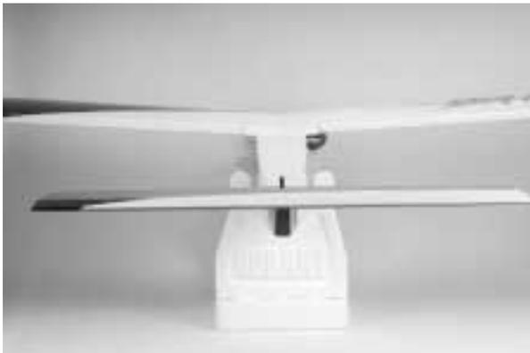
**6.** When you're satisfied with the alignment, use a pencil to carefully trace around the bottom of the stabilizer where it meets the fuselage.
