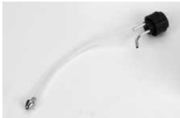
8. Carefully insert the assembly into the fuel tank and, using the self-tapping screw, screw the stopper together firmly. It helps if the screw has been inserted in the assembly and started — then insert the assembly into the tank and tighten the screw so the stopper is snug in the tank. As the screw is tightened, the stopper parts come together, compressing the rubber stopper snugly inside the throat of the tank.
