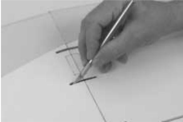
**8.** Trial fit the aileron tray supports into the slots. It may be necessary to enlarge the slots slightly to accommodate the supports.
