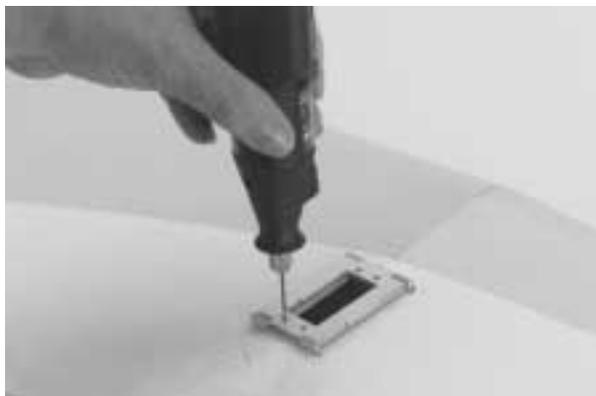
3. Place the aileron servo back in its mount in the wing and secure it in place using the four screws included with the servo.
