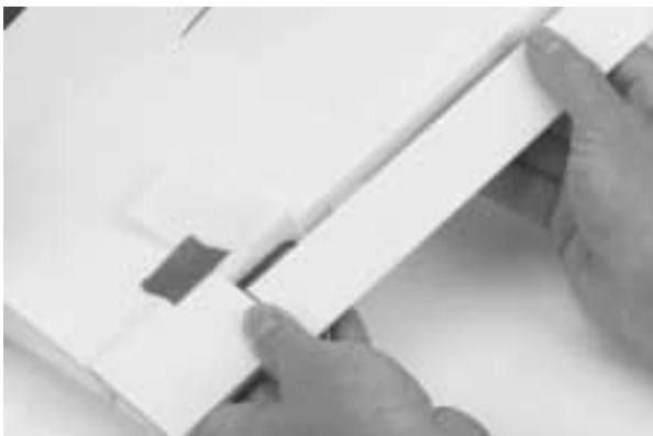
**8.** Carefully wipe off any excess epoxy using a paper towel and rubbing alcohol.
