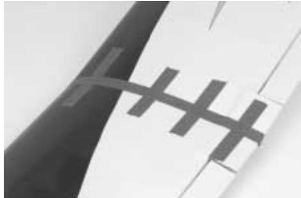
**17.** Apply masking tape at the wing joint to hold the wing together securely while the epoxy cures. Place the wing on a large, flat surface. With one wing panel lying flat on the surface, the opposite wing tip should be propped up exactly  $4\frac{1}{2}$ " from the surface. Allow the wing joint to dry overnight.
