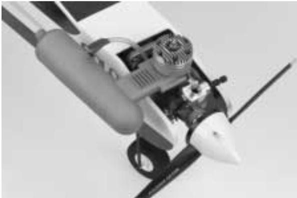
**2.** Connect the vent tube from the fuel tank to the pressure fitting on the muffler. Remove the masking tape at this time.
