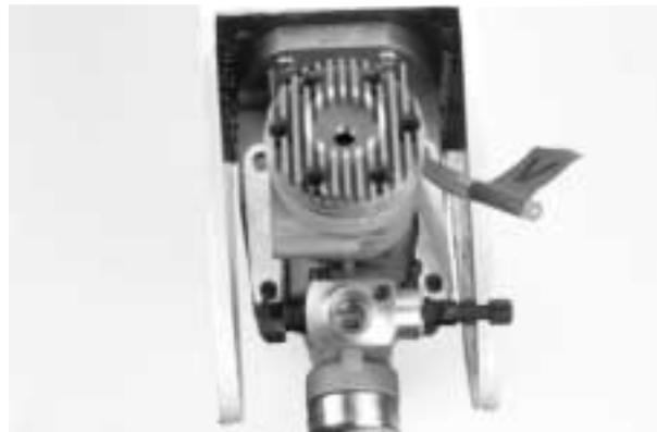
**4.** Insert one 4x20mm screw into each of the engine mounting bracket holes. Press one of the 4mm nuts into the corresponding receptacles on the bottom of the motor mount. Apply thread lock to secure the nut in place and firmly tighten the screw. Repeat the procedure for the other three screws.
