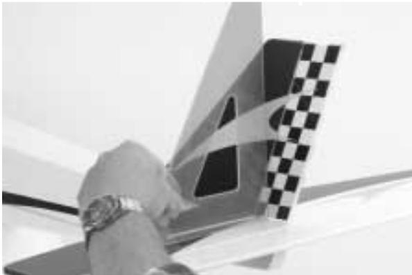
**12.** Using a pencil, trace around the vertical stabilizer where it meets the fuselage. Again, the pencil should leave a light indentation in the covering of the vertical stabilizer.
