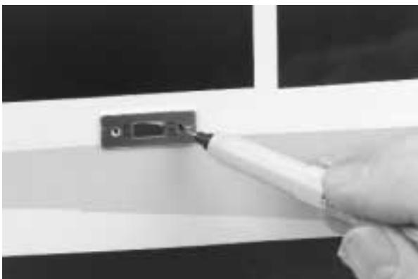
**10.** Remove the switch plate from the fuselage. Drill the two mounting holes as marked using a 1/16" drill bit.
